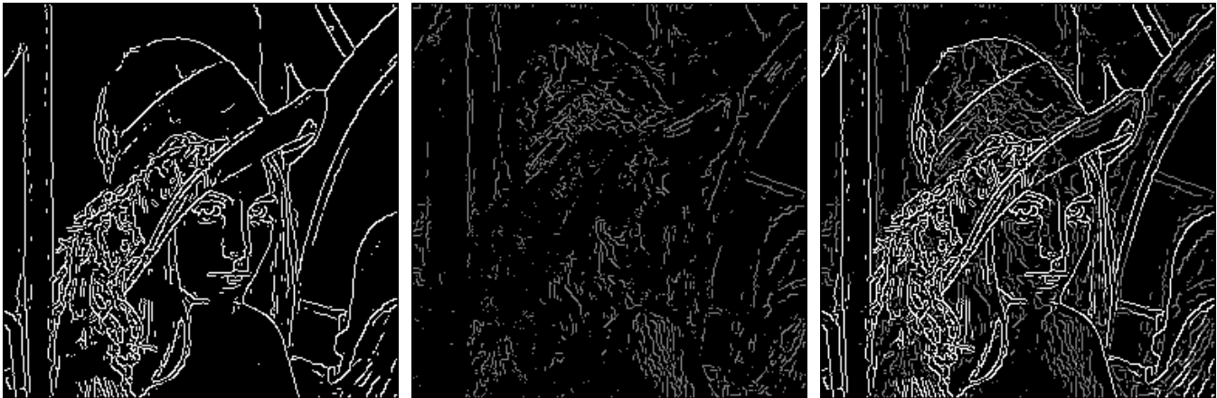
Figure P.11: Step 4: Double threshold. The strong pixels (left), the weak pixels (middle), and the combined (right).
